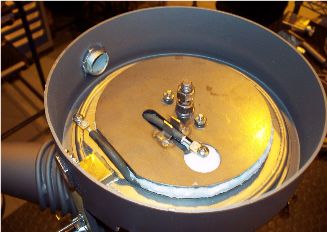
Figure 3-7 VHS-4, VHS-6 and VHS-250 Heater Mounting (VHS-6 Shown)
